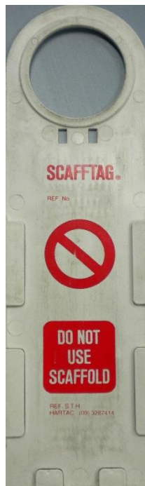
Scaffold tag holder depicting that the scaffold is unsafe for use
