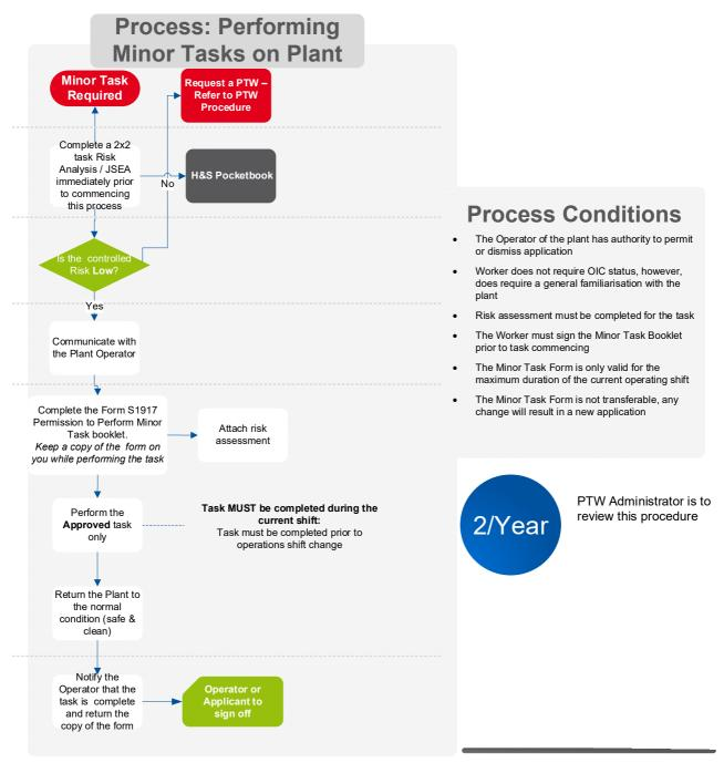
Process: Performing Minor Tasks on Plant
