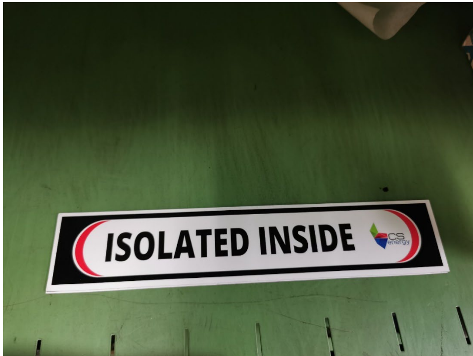
Magnetic Sign used for awareness when Isolations are installed inside a cabinet
