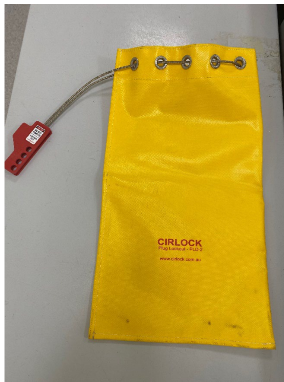
Plug Lockout Bag – Power or Hose Isolations
