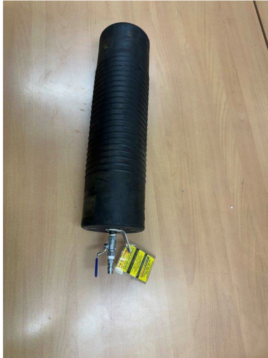
Isolation of spooling where valves are not present
