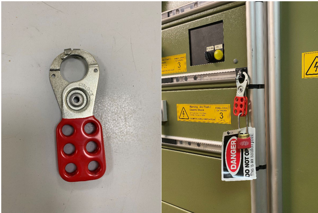
Metal Hasp – Not to be used in electrically conductive environment. Multiple uses for isolations and also useful for multiple locks on a single point
