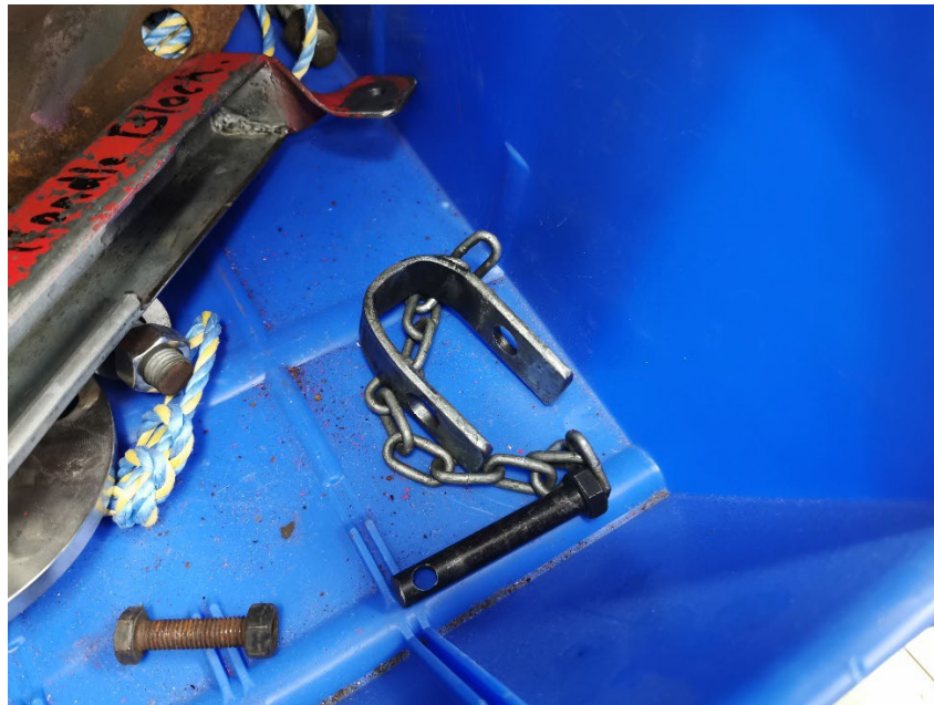
Custom Device for use on Callide B Turbine Reset Lever
