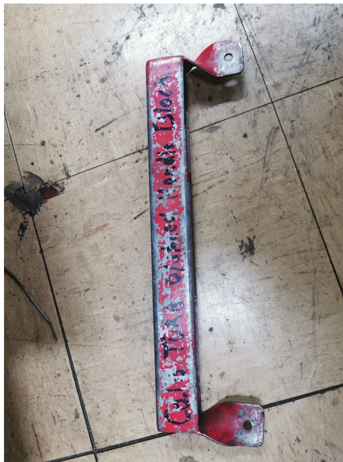
Custom Device for use on Callide B Turbine Trip Lever
