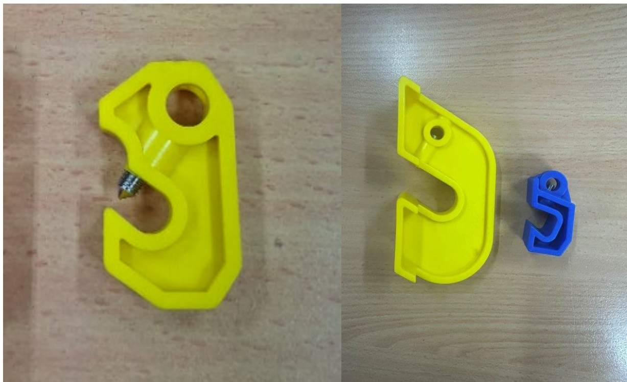
Alternative Style Lock out device / clamp for Circuit Breakers
