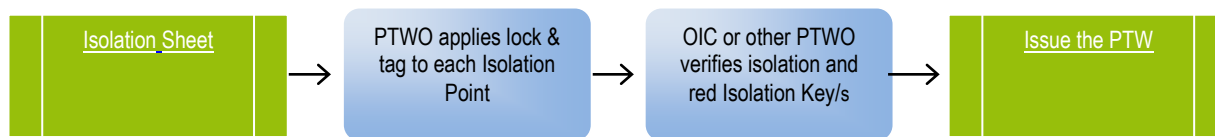
Figure: 4.2 Isolating the Plant
