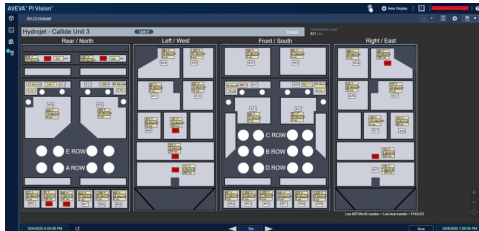
Figure 13 - 9 Red Zones Indicating Clinker Growth from PI Vision on 3 April 2025, 19:00 Handover
