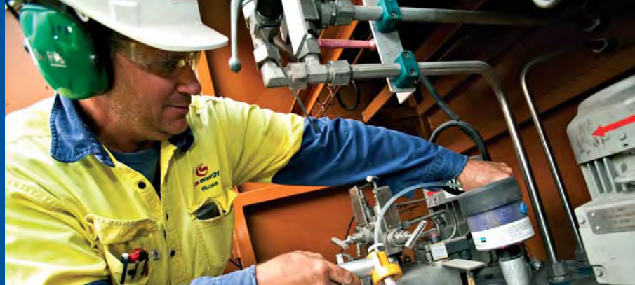
Ross Morrish, Utility Worker, taking oil samples for testing under the lubrication standards
